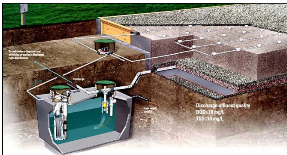
FIGURE 6.3 Typical Recirculating Sand Filter
